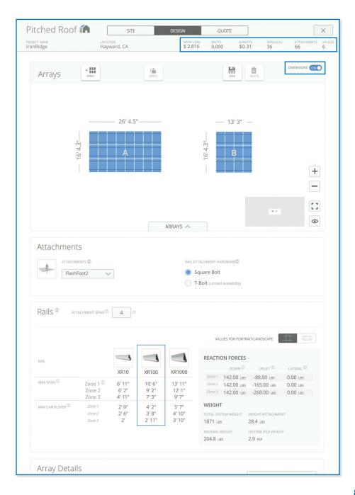
Module orientation will impact how many solar panels can fit into a single continuous row. Modules are most commonly installed in portrait orientation as it allows more modules to be placed in a single row which helps save on material costs.
