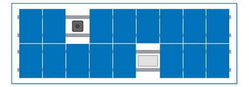
In this scenario, you will not want to remove modules from the Array Editor. Instead, you should design the project as though the modules will remain – which will ensure that you have enough rail. When you complete your project design and move onto the "Quote" tab, you can manually add one kit of Stopper Sleeves (to transform the UFO into an end clamp) for each obstruction spanned over.
