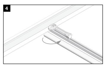
Rotate handle with an upwards motion until CAMO<sup>®</sup> snaps into rail channel. Ensure Camo bonding pins are fully seated on top of module frame.
