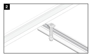
Place module on rails (module cells not shown for clarity).
