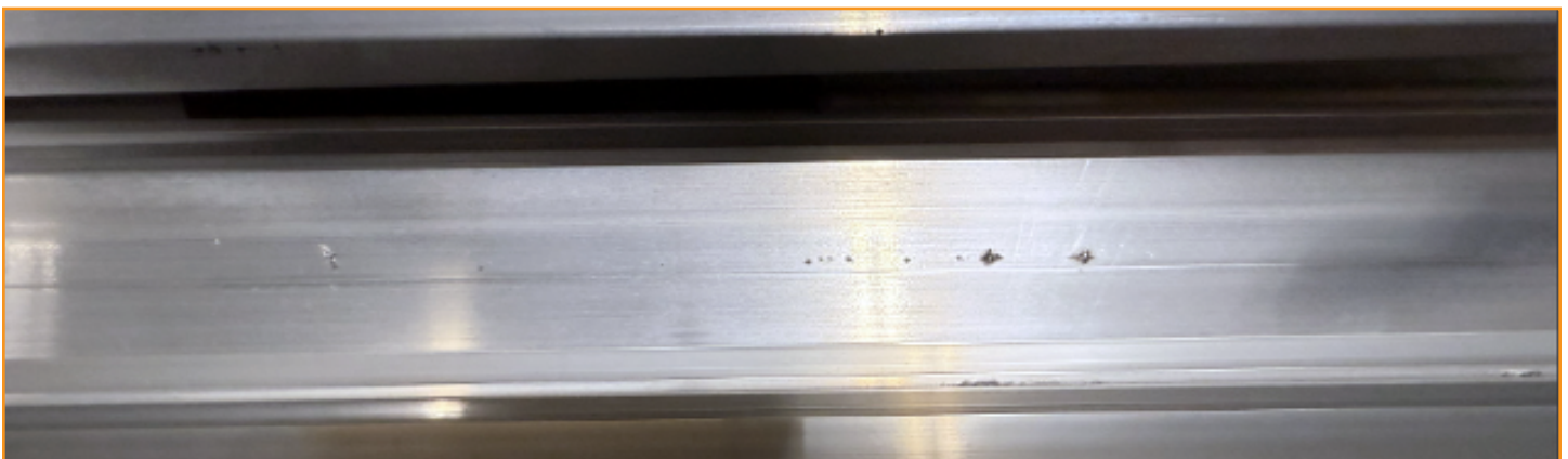
Spotches showing on an unfinished, mill stick of aluminum rail.
