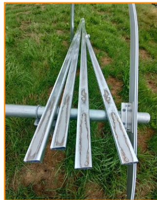
Visible stains on mill rails.
