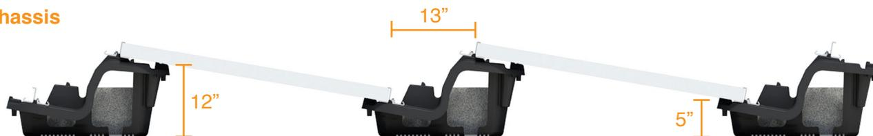
With 10-13" inter-row spacing, BX provides an **8-10% increase** in power density compared with other ballasted systems—that's a **capacity increase of 20%** in a typical 50kW system. The BX Chassis geometry also offers more than 5" of clearance in the 10-degree configuration and 8" in the 5-degree configuration, enabling the system to avoid drain domes, roof saddles, and conduit supports.
