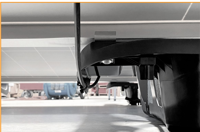
Examples of wire installation under BX Chassis.
