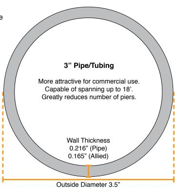
Refer to the following table to see how size impacts the East-West span between foundations. The table complies with ASCE 7-10 structural code. Values are based on 72-cell modules in Wind Exposure Category B.
