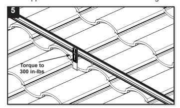
Attach rails to either side of slot using bonding hardware. Level rails at desired height. Ensure hook does not extend beyond top of rail surface. Torque hardware to 300 in-lbs (25 ft-lbs).
