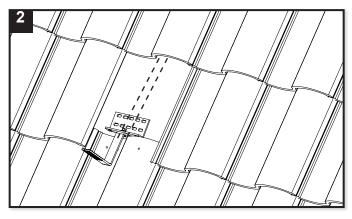
Position base over rafter, adjust arm if necessary and torque hardware to 132 in-lbs. Position arm near center of valley for curved tiles.
