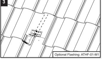
Use base as guide to drill 1/4" pilot holes, then fill with roofing manufacturer's approved sealant. Insert lag bolts and tighten until fully seated. IronRidge offers an optional aluminum deck flashing. Other approved flashing methods include user supplied adhesive backed flexible flashing.
