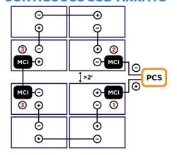
Where any string is connected across non-contiguous sub-arrays separated by more than 2' (see example figure), MCI-1s shall be installed as follows:
