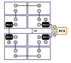
Where any string is connected across noncontiguous sub-arrays separated by more than 2' (see example figure), MCI-2s shall be installed as follows:
