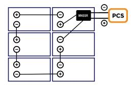
Where one or more PV strings are connected within a single contiguous array as shown in the figure, the positive and negative ends of each string shall be connected to the MNSSR. The leads of each MNSSR get connected to the PCS. If there are multiple arrays, then each array each shall be equipped with an MNSSR as shown in the figure.
