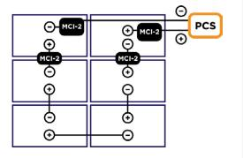
Where one or more PV strings are connected within a single contiguous array as shown in the figure, Tesla MCI-2s shall at a minimum be installed at both the positive and negative ends of each string between the last module and the homerun to the PCS. Two more MCI-2s are required anywhere within the string, but suggested to be placed between near ends of each string as shown in figure above.
