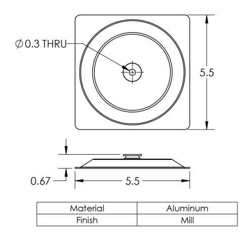
3) WASHER, SEALING, 5/16" EPDM BACKED STAINLESS STEEL
