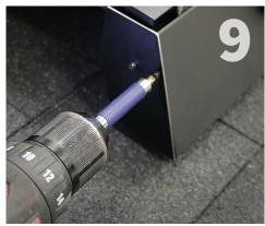
Attach End Caps with the provided screws, screwing through the holes on the end cap with a #2 Phillips screwdriver, into the screw bosses of the extrusion insuring the black side of the Skirt End Caps is facing outward.
