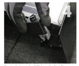
To attach, insert the QClick on the End Clamp at a slight angle into the channel on the QSkirt. While holding firmly in place, rock the QClick until it clicks into place.
